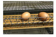
•Holed: polyester material, has a larger elongation than the solid egg collecting belt. After a period of use, the belt has to be cut short and stitched again. If egg is broken, the egg liquid can flow into the feed trough below the belt through these holes to reduce effect.
