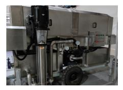
Vertical multistage centrifugal pump, high lift/high pressure/good cleaning effect
